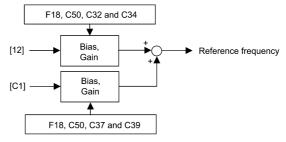
In the case of unipolar input (terminal [12] with C35 = 1, terminal [C1], terminal [V2] with C45 = 1)
