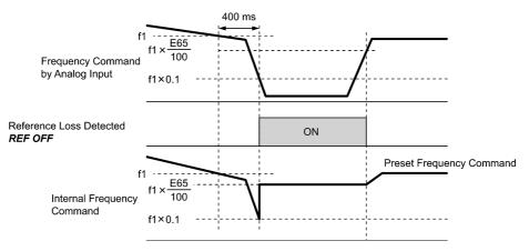
In the diagram above, fl is the level of the analog frequency command sampled at any given time. The sampling is repeated at regular intervals to continually monitor the wiring connection of the analog frequency command.
