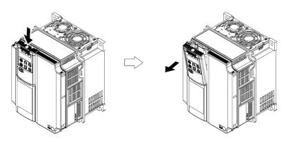
Figure 2.22 Removing a Keypad
