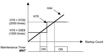
To enable this function, assign the maintenance timer signal MNT to one of the digital output terminals (function code data = 84).
