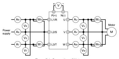
Figure 7.1 Connection of Meters
