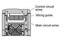
Control circuit wires
