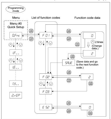
Figure 3.2 Menu Transition in Menu #0 "Quick Setup" and Function Code Data Changing Procedure
