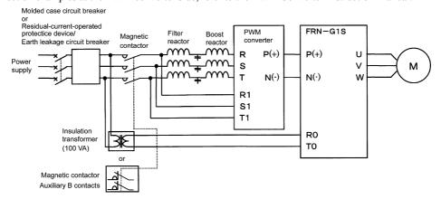
Figure 2.9 Connection Example of PWM Converter
