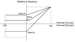
A reference frequency can be specified not only with the frequency (Hz) but also with other menu items, (Note depending on the setting of function code E48 (= 3 to 5, or 7).
