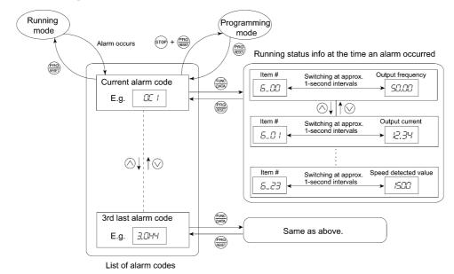
Figure 3.7 Menu Transition in Alarm Mode
