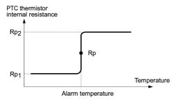
Suppose that the internal resistance of the PTC thermistor at the alarm temperature is Rp, the detection level (voltage)  $V_{v2}$  is calculated by the expression below. Set the result  $V_{v2}$  to function code H27.
