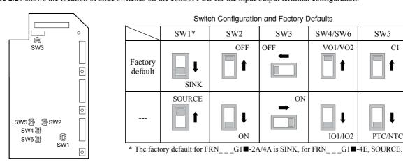
Figure 2.20 Location of the Slide Switches on the Control PCB
