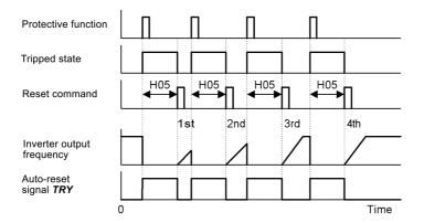
In the figure below, the inverter failed to restart normal operation within the number of reset times specified by H04 (in this case, 3 times (H04 = 3)), and issued the alarm output (for any alarm) **ALM**.
