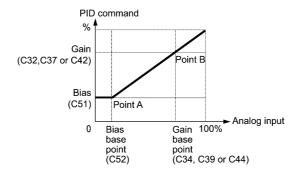
(Example) Mapping the range of 1 through 5 V at terminal [12] to 0 through 100%
