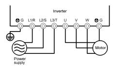
Figure 4.2 Connection of Main Circuit Terminals
