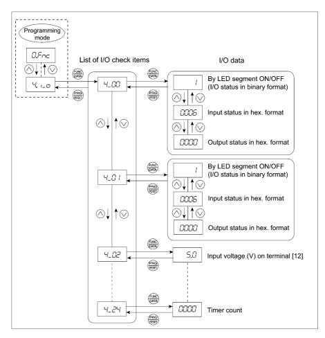
Figure 3.4 Menu Transition in Menu #4 "I/O Checking"
