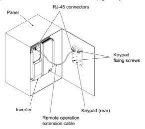
Figure 2.21 Mounting a Keypad on the Panel Wall
