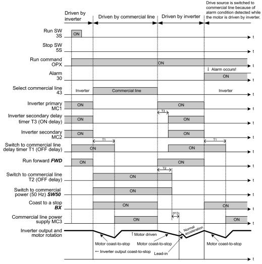
Alternatively, you may use the integrated sequence by which some of the actions above are automatically performed by the inverter itself. For details, refer to the description of *ISW50* and *ISW60*.
