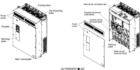
Figure 1.2 Outside and Inside Views of Inverters
