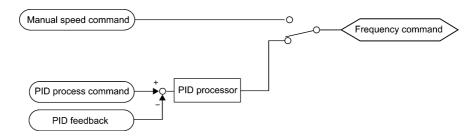
PID process control block diagram
