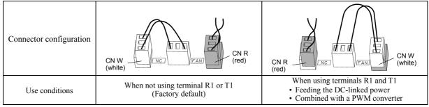
Note: A box (■) in the above figure replaces S or E depending on the enclosure.
