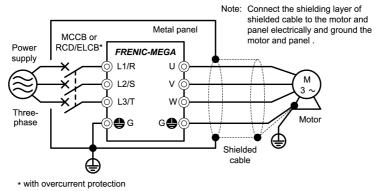
Figure 9.2 Mounting the Inverter in a Metal Panel
