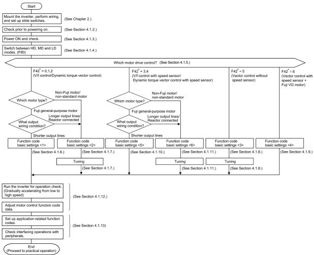
Figure 4.1 Test Run Procedure
