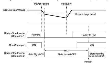
**Factory default:** By factory default, H13 is set to the value suitable for the standard motor (see Table B in Section 5.1 "Function Code Tables"). Basically, it is not necessary to change H13 data. However, if the long restart time causes the flow rate of the pump to overly decrease or causes any other problem, you might as well reduce the setting to about a half of the default value. In such a case, make sure that no alarm occurs.
