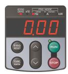
Figure 4.3 Display of the LED Monitor after Power-on
