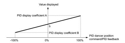
If the sensor output is unipolar, the PID dancer control operates within the range from 0 to  $\pm 100\%$ , so virtually specify the value at  $\pm 100\%$  as coefficient B.
