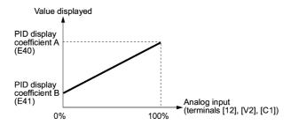
To set up the analog input monitor, use function codes E61 through E63. Use E43 to choose the item to be displayed.
