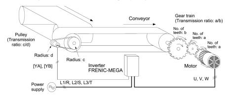
An Example of a Closed Loop Speed Control System (Conveyor)
